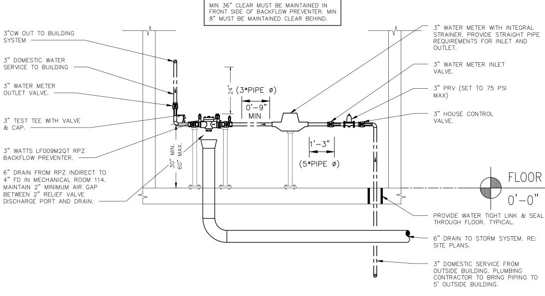
PLUMBING ELEVATION A-A SCALE: 1/2" = 1'-0
