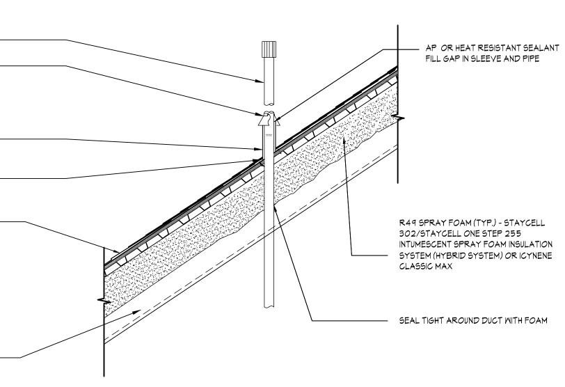
METAL DUCT / PIPE SEE MEP DOCUMENTS METAL PIPE HOOD WITH COLLAR AND AP OR HEAT RESISTANT SEALANT
