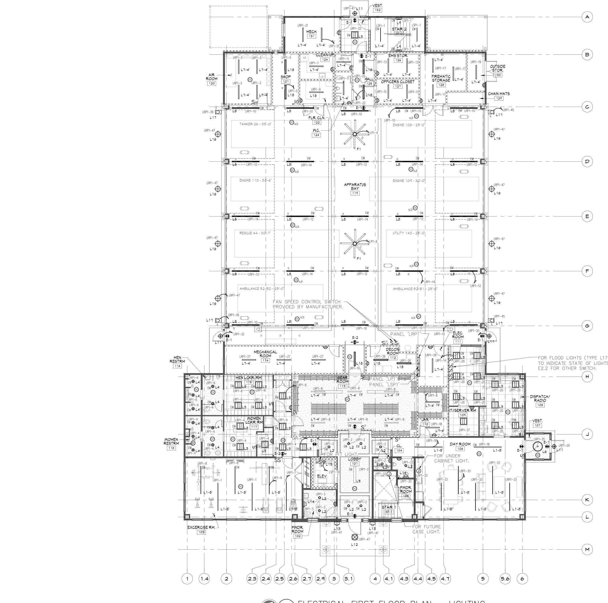
ELECTRICAL FIRST FLOOR PLAN – LIGHTING SCALE: 1/8" = 1'-0"
