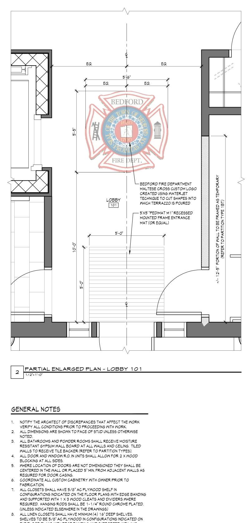
SHELVES TO BE 5/8" AC PLYWOOD IN CONFIGURATIONS INDICATED C THE FLOOR PLANS WITH EDGE BANDING AND SUPPORTED WITH 1X3 WOOD CLEATS AND DIVIDERS WHERE REQUIRED.
