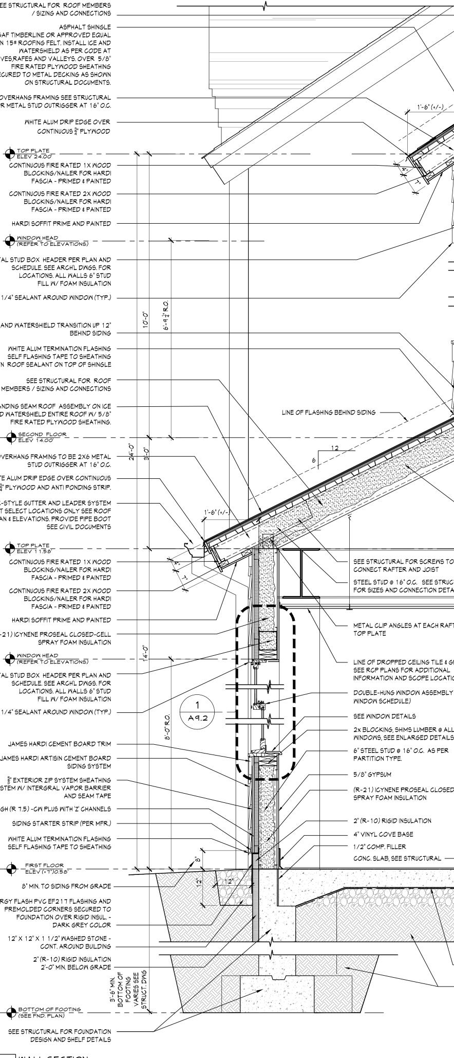
SEE STRUCTURAL FOR ROOF MEMBERS / SIZING AND CONNECTIONS
