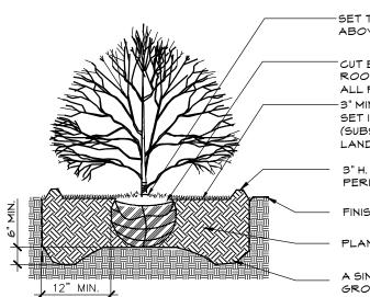
SET TOP OF ROOTBALL AT OR SLIGHTLY ABOVE GRADE WHERE PLANT WAS DUG CUT BURLAP & TWINE FROM TOP = OF ROOTBALL; LOOSEN ALL TIES, REMOVE ALL PLANT TAGS 3" MIN SHREDDED CEDAR F SET IN 3" DEEP WATERING SAUCER (SUBSTITUTES APPROVED BY
