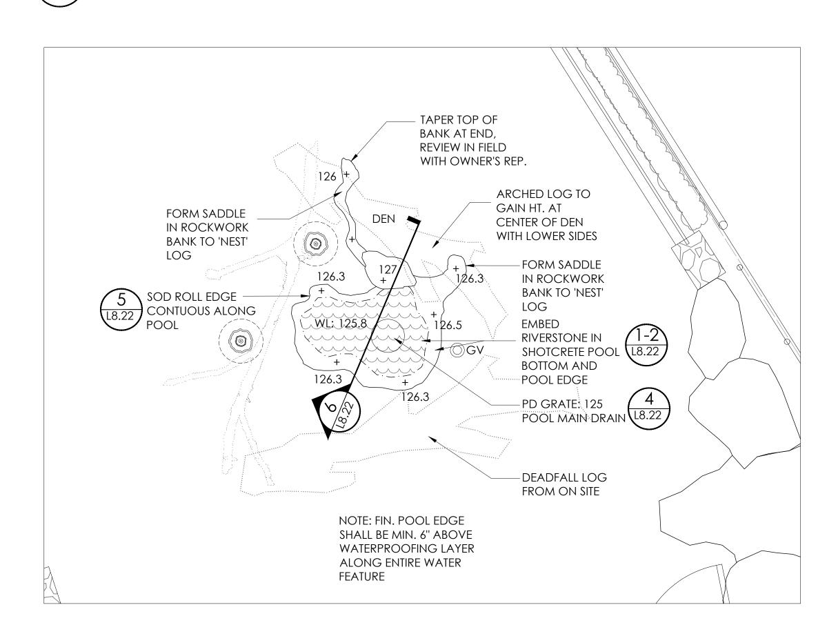
DETAILED LAYOUT PLAN PORCUPINE DRINKING POOL & DEN 2 DETAILED LAY SCALE: 1/2" = 1'-0"
