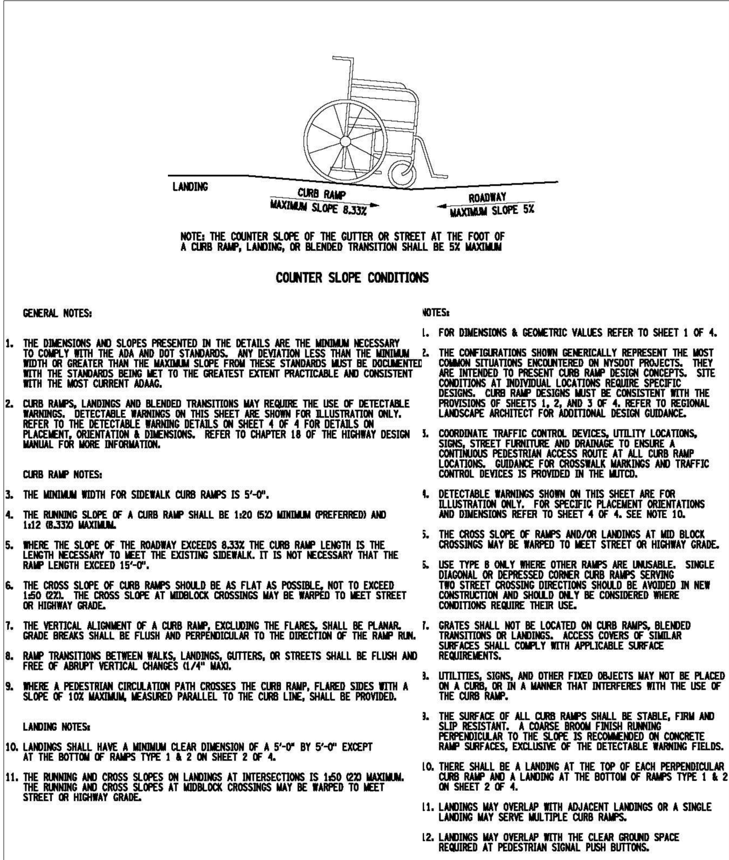
SIDEWALK CURB RAMP NOTES N.T.S.
