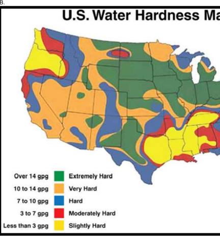
RECOMMEND BI-ANNUAL FLUSHING OF TANKLESS HEAT EXCHANGER IN AREAS WATER IS GREATER THAN 10GPG. REFERENCE RINNAI WATER HEATER INSTALL OPERATION MANUAL FOR INSTRUCTIONS
