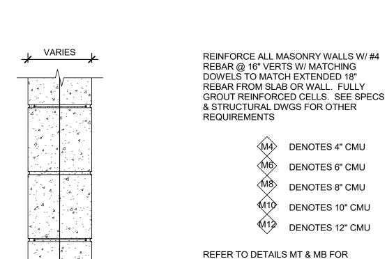
CONCRETE MASONRY UNIT WALL
