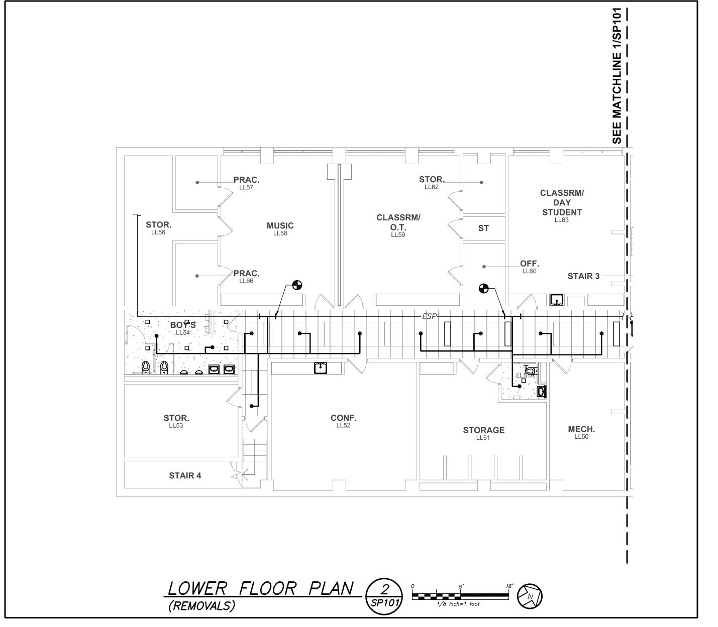
REMOVE EXISTING SPRINKLER HEADS AND BRANCH PIPING IN ALL AREAS CEILINGS ARE TO BE REPLACED. PROVIDE NEW HEADS AND CONNECT TO EXISTING BRANCH PIPING.
