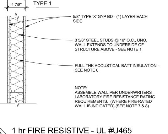
(FOR TYPE 1A - USE 6" STEEL STUDS) (FOR TYPE 1B - USE 8" STEEL STUDS)
