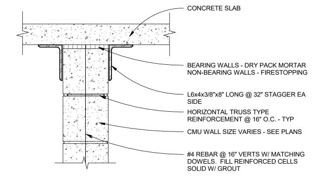
TYPICAL CONCRETE MASONRY MT UNIT WALL / SLAB ATTACHMENT
