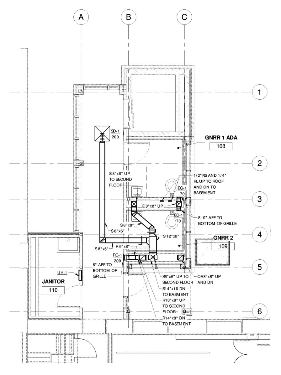
FIRST FLOOR HVAC PLAN SCALE: 1/4" = 1'-0"
