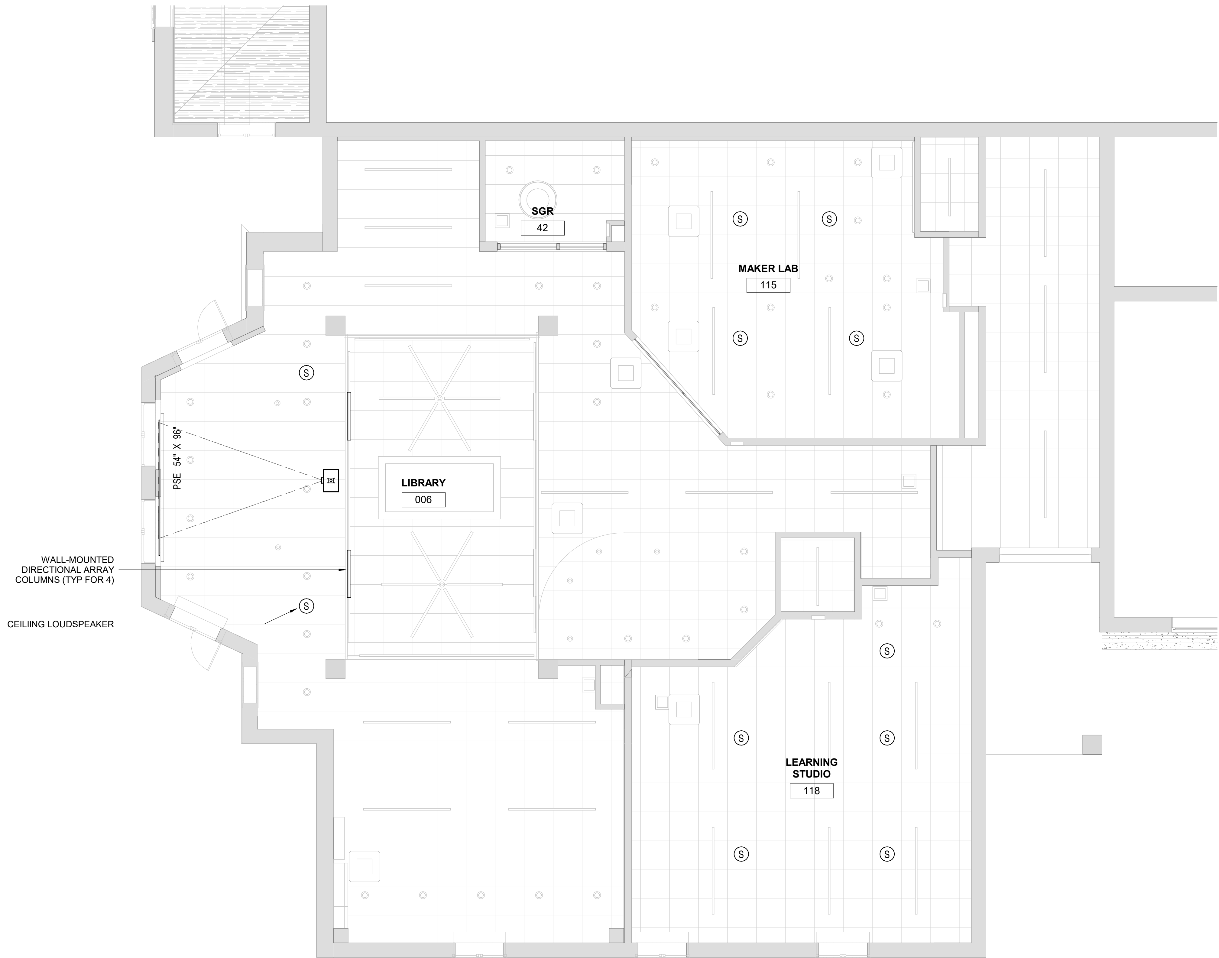
1 AUDIOVISUAL FIRST FLOOR REFLECTED CEILING PLAN - LIBRARY 1/4" = 1'-0"
