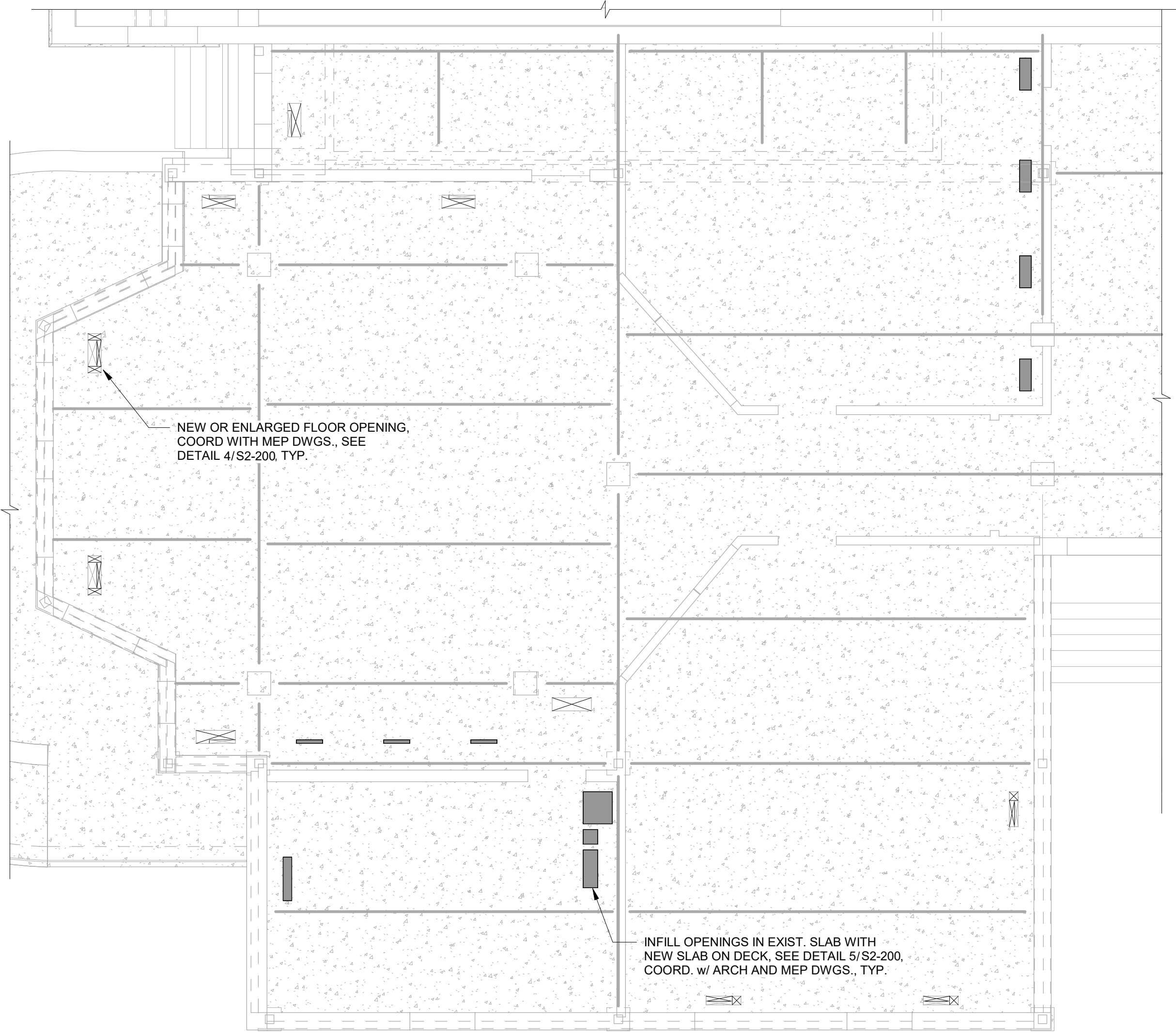
1 PARTIAL FIRST FLOOR FRAMING PLAN SCALE: 3/16" = 1'-0"
