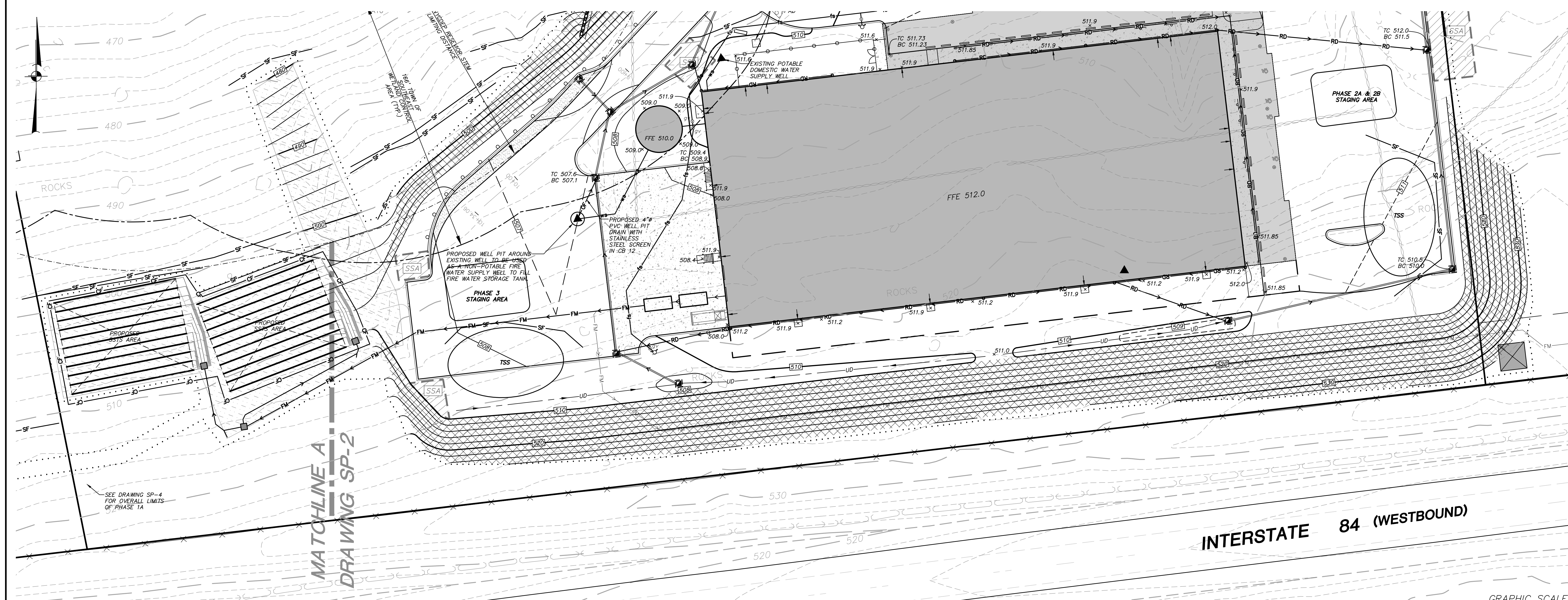
GRADING, UTILITIES, AND EROSION CONTROL FOR SSTS
