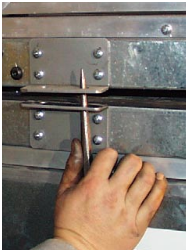
FIG. 2-18 – GUIDING BRACKETS TOGETHER
