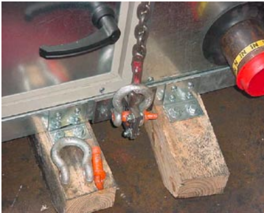
FIG. 1-5 – PROPER LIFTING WITH SHACKLE AND HOOK AT LIFTING LUG
