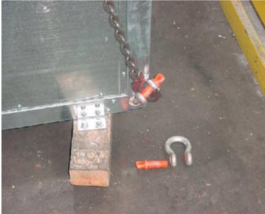
FIG. 1-4 – PROPER LIFTING WITH SHACKLE AND HOOK AT CORNER
