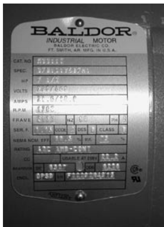
FIG. 2-21 – TYPICAL MOTOR DATA / NAMEPLATE
