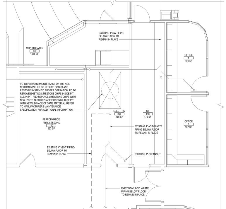
ACID NEUTRALIZING PIT - PROPOSED WORK
