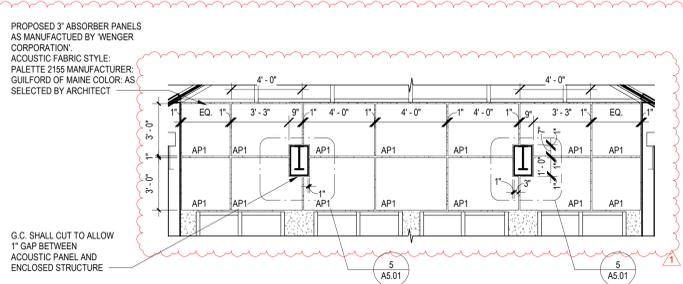
**6 ACOUSTIC PANEL INTERIOR ELEVATION A - (TYPICAL 2 ELEVATIONS)**
