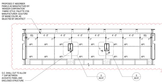
**7 ACOUSTIC PANEL INTERIOR ELEVATION B - (TYPICAL 2 ELEVATIONS)**
