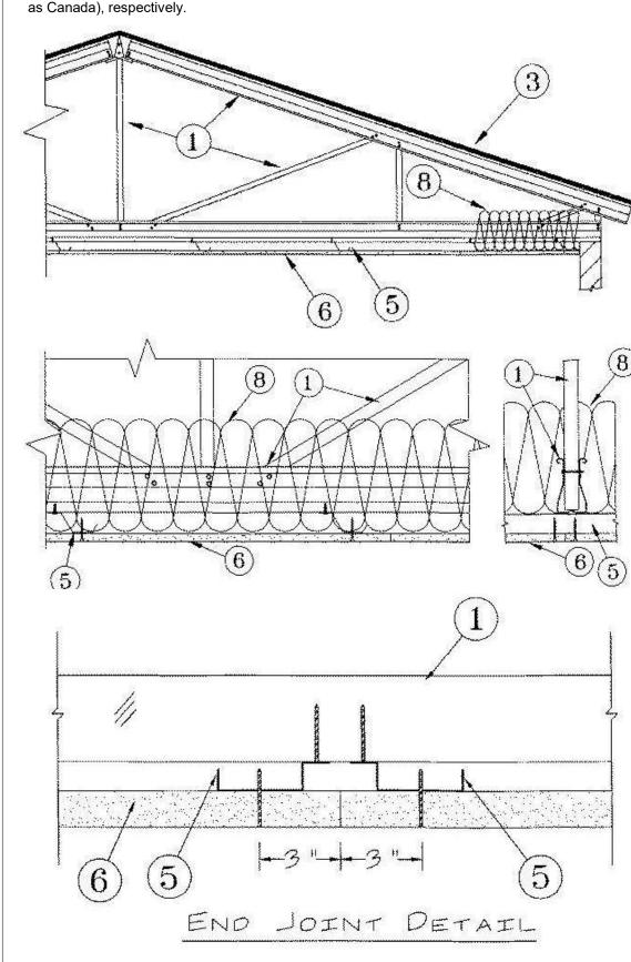
1. Structural Steel Members\* — Pre-fabricated light gauge steel truss system consisting of cold-formed, galv steel chord and web sections. Trusses fabricated in various sizes, depths and from various steel thickness, Trusses spaced a max of 24 or 48 in. OC, See Item 3. TRUSSTEEL, DIV OF ITW BUILDING COMPONENTS INC — TrusSteel
