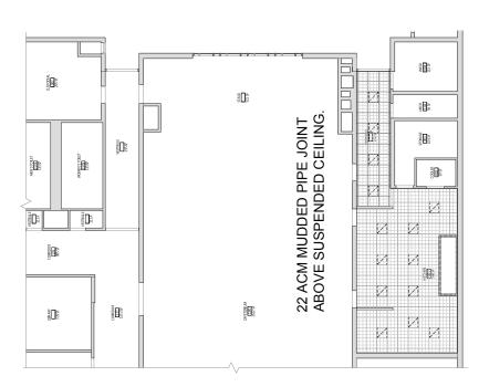
$2 \atop_{\text{HAZ101}}$  kitchen - Demolition reflected ceiling plan
