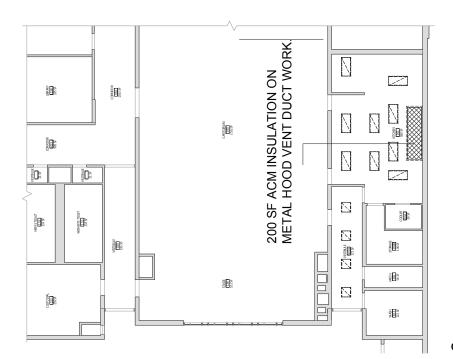
$\sum_{\text{FAZ101}} \text{KITCHEN}$  - DEMOLITION REFLECTED CEILING PLAN
