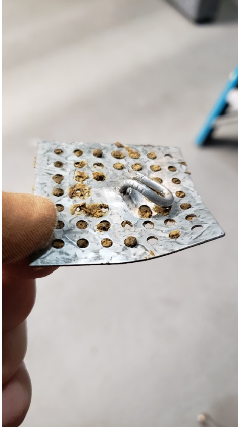
Asbestos containing Mastic to Fiberglass Duct Insulation Clamps, Brown
