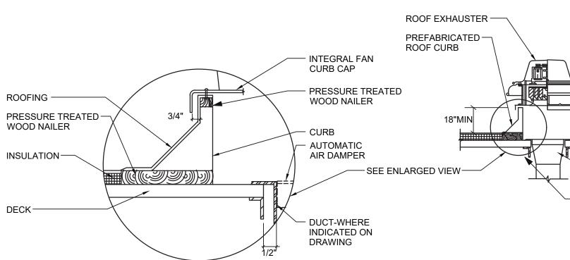
MECHANICAL DUCT CONSTRUCTION DETAIL M-82 / SCALE: NOT TO SCALE
