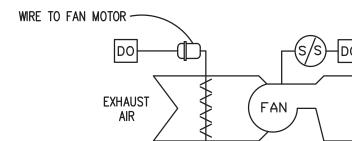
EXHAUST FAN - CONSTANT SPEED - SEQUENCE OF OPERATIONS:
