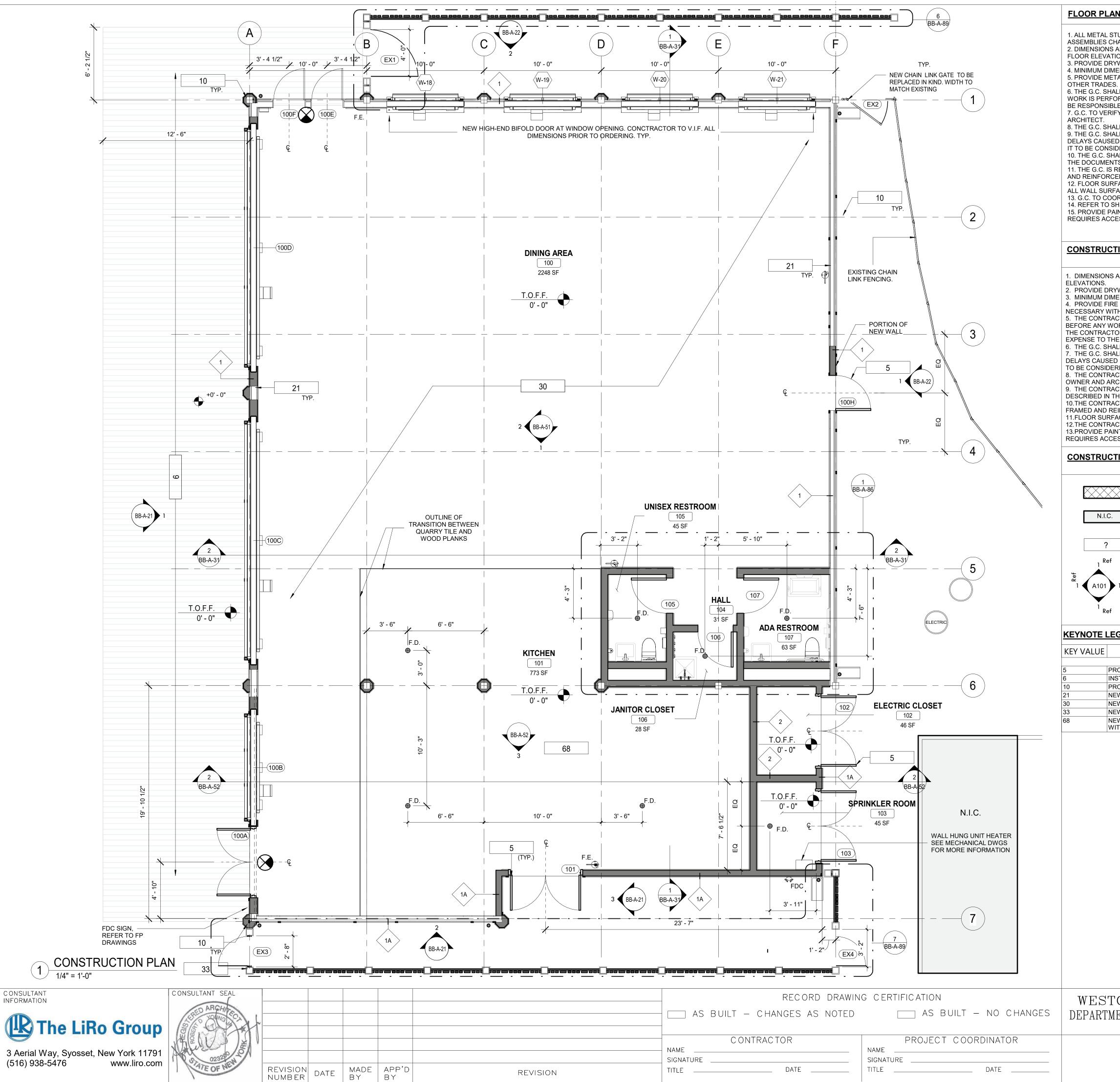
1. ALL METAL STUDS 20 GA- TYPICAL NON-LOAD BEARING PARTITIONS. SEE USG STEEL- FRAMED DRYWALL SYSTEMS " LIMITING HEIGHT"- STEEL STUD
