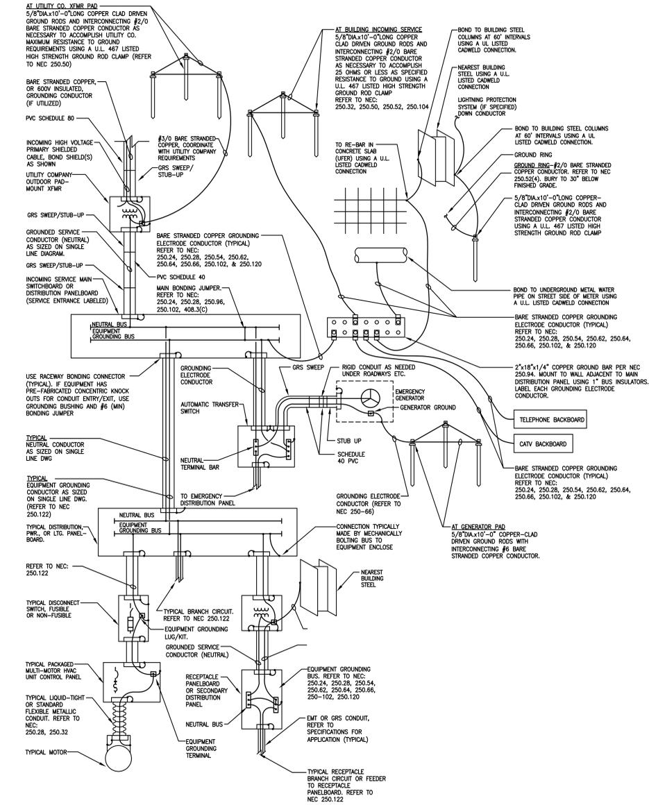
**SYSTEM GROUNDING AND BONDING DIAGRAM**
