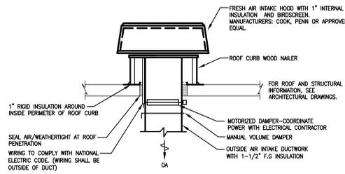
**ROOF FRESH AIR INTAKE DETAIL**
