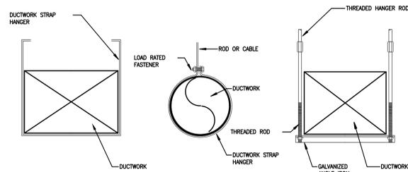
**DUCTWORK HANGER DETAIL**
