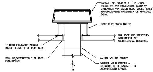
**ROOF EXHAUST AIR HOOD DETAIL**
