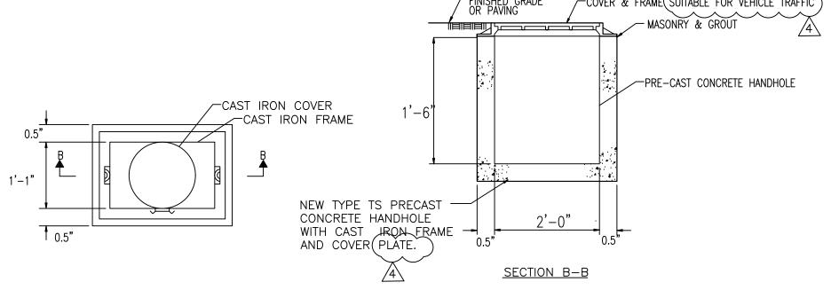
ELECTRICAL HANDHOLE DETAIL SCALE: NTS (VEHICLE TRAFFIC RATED)
