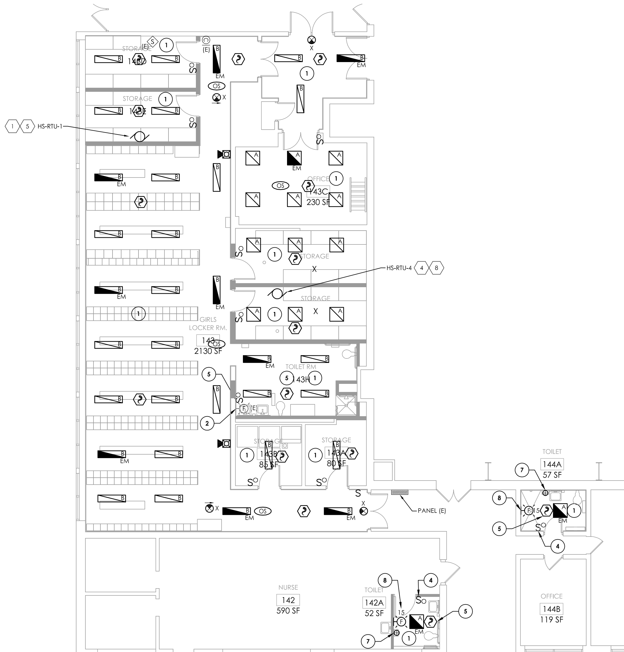
1 FIRST FLOOR ELECTRICAL NEW WORK PLAN SCALE: 1/8" = 1'-0"
