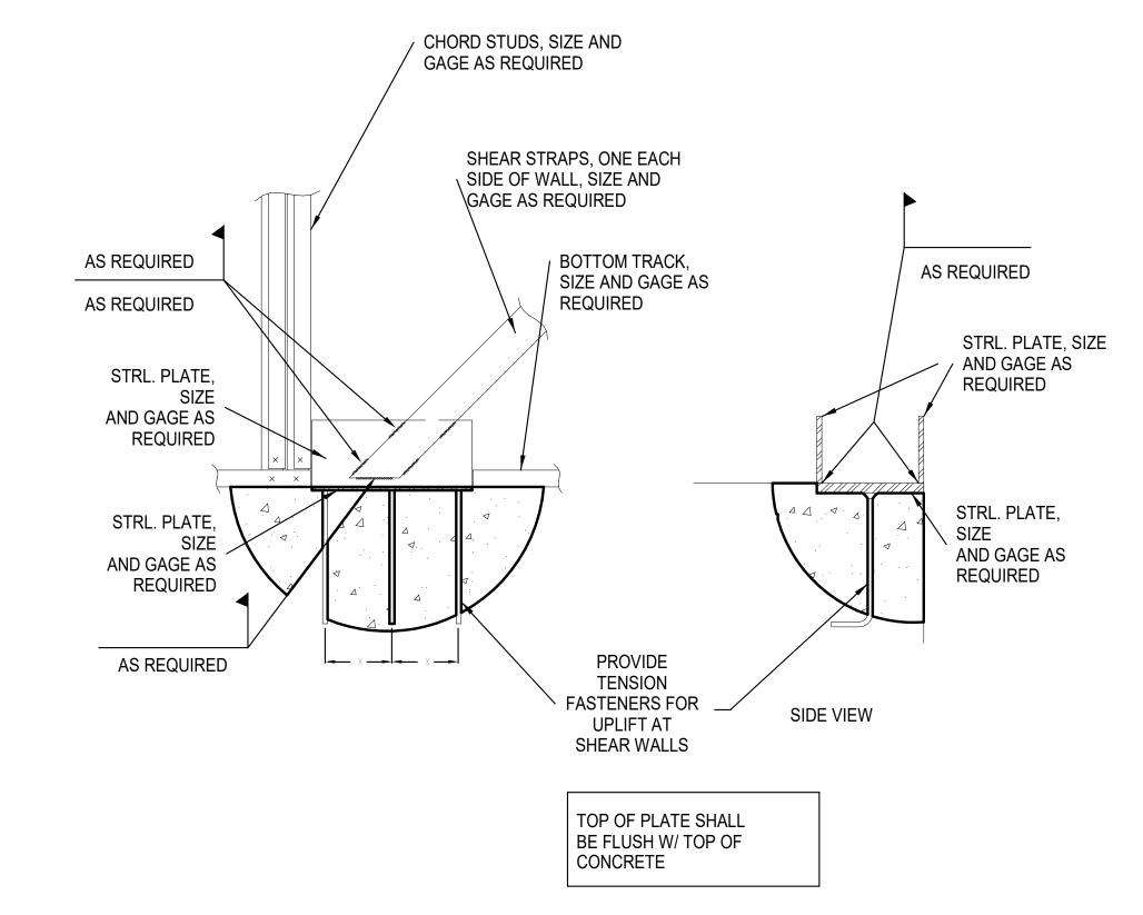
3 TYPICAL SHEAR WALL STRAP AT BASE
