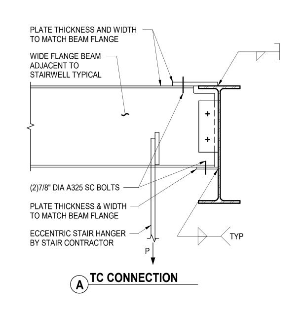
PLATE THICKNESS AND WIDTH TO MATCH BEAM FLANGE WIDE FLANGE BEAM ADJACENT TO STAIRWELL TYPICAL 3/8" FITTED STIFFENER WHERE INDICATED AS TCS MATCH FAR SIDE STIFFENER WHERE FITTED VERTICAL STIFFENER OCCURS (2)7/8" DIA A325 SC BOLTS PLATE THICKNESS & WIDTH -ECCENTRIC STAIR HANGER TO MATCH BEAM FLANGE BEYOND BY STAIR CONTRACTOR TCS CONNECTION
