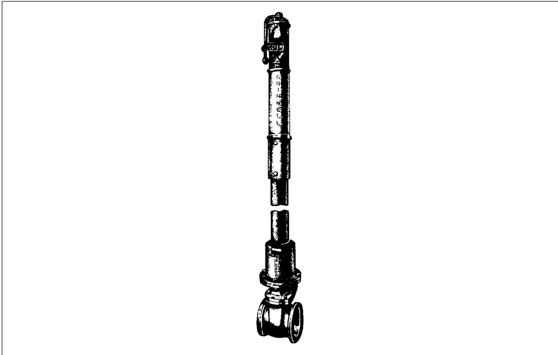
Fig. 3.1.1.6.4-1. Gate valve with indicator post
