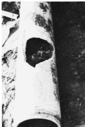
Fig. 3.1.9.2.1-1. Examples of low pressure hydro breaks
