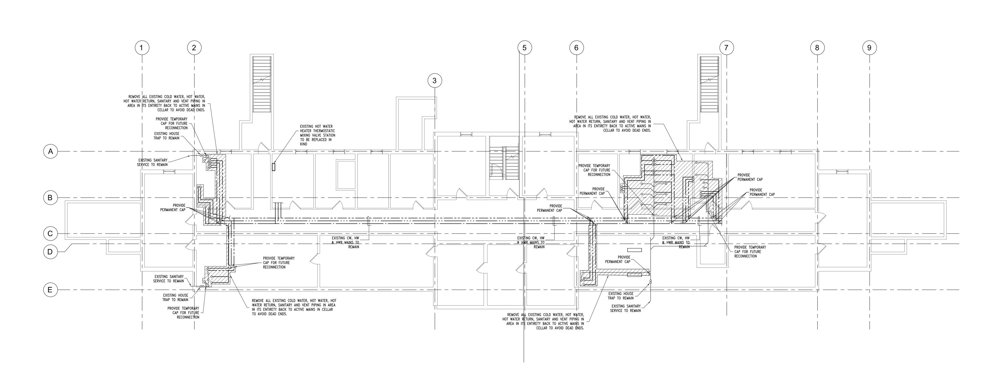
1. PLUMBING CONTRACTOR TO SHUT-OFF, DISCONNECT, CUT AND CAP, OR OTHERWISE SECURE UTILITIES PRIOR TO DEMOLITION WORK BY GENERAL CONTRACTOR. GENERAL CONTRACTOR TO CONFIRM UTILITIES DISCONNECTED AND SECURED PRIOR TO REMOVALS.
