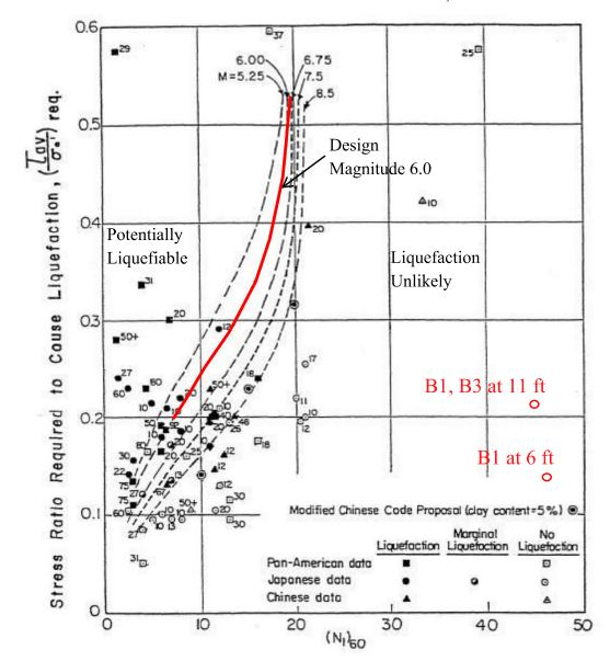
Figure 16 Relationship between stress ratios required to cause liquefaction and (N<sub>1</sub>)<sub>60</sub> values for cohesionless soils having fines content of 35% in M=5.25-8.5 earthquakes (Seed et al., 1985)
