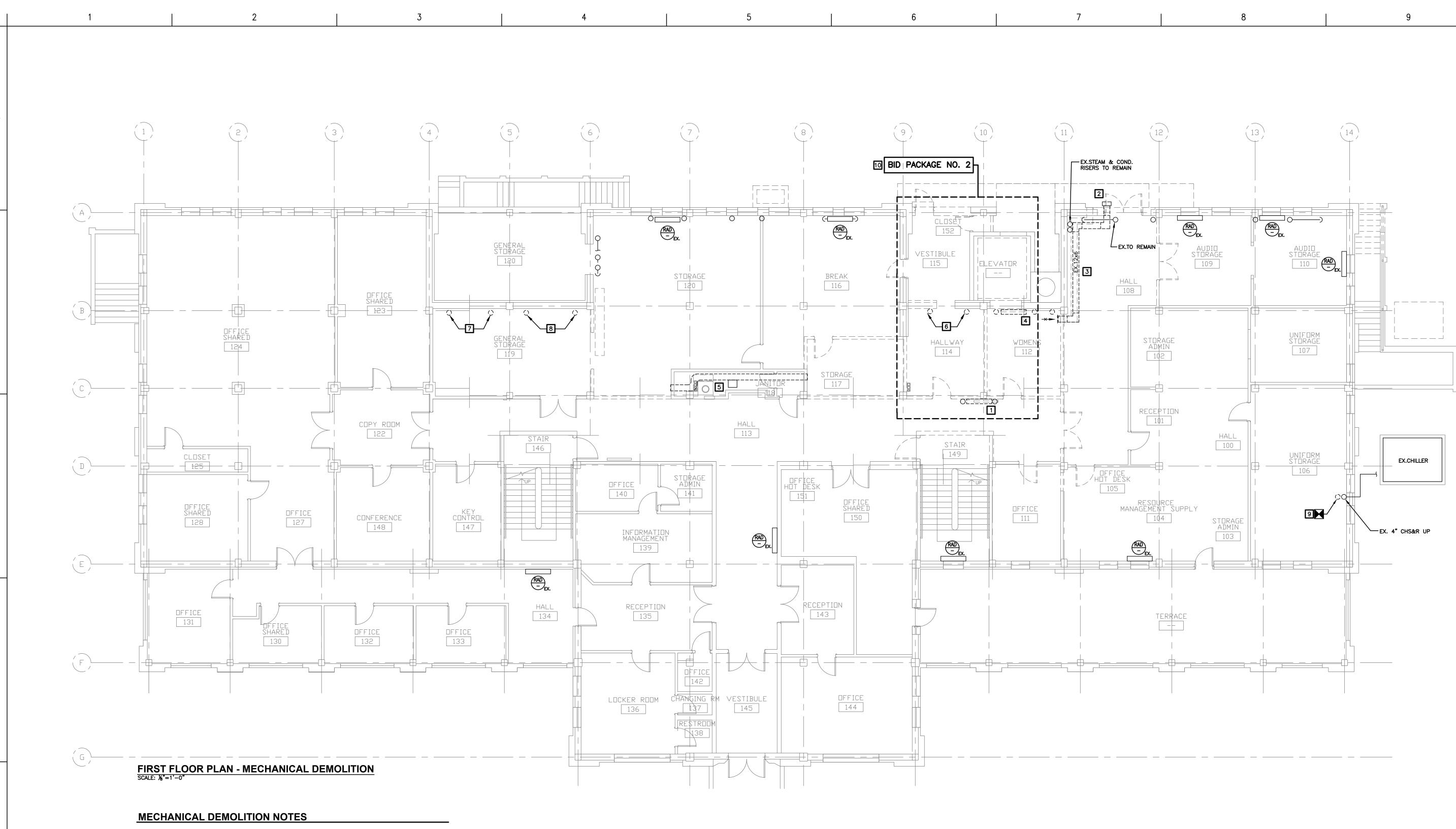
1 REMOVE EX. RADIATOR. CAP STEAM AND CONDENSATE PIPING NEAR MAINS ON FLOOR BELOW. RADIATOR TO BE RELOCATED TO NEW LOBBY 112. REFER TO NEW WORK PLAN.
