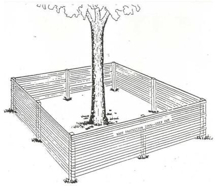
**DETAIL A** <u>Pre-Construction Barricade Fencing</u> four (4) foot high, orange polyethylene barricade fence supported on postswith attachments to these posts on six (6) foot centers.
