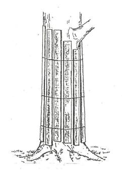
**DETAIL B** Boards or poles lashed with rope or wire in an upright position against thetree trunk.
