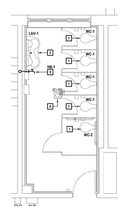
1 First Floor Girl's Bathroom Construction Plan
