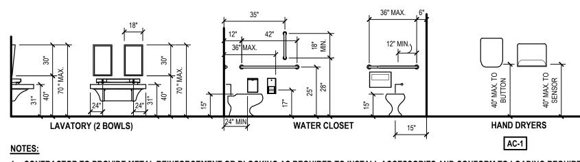
1. CONTRACTOR TO PROVIDE METAL REINFORCEMENT OR BLOCKING AS REQUIRED TO INSTALL ACCESSORIES AND CONFORM TO LOADING REQUIREMENTS. 2. INSULATE DRAINAGE AND SUPPLY PIPES BELOW ALL SINKS (TYP.) MATERIALS PROVIDED BY GENERAL CONSTRUCTION CONTRACTOR, INSTALLED BY PLUMBING CONTRACTOR.
