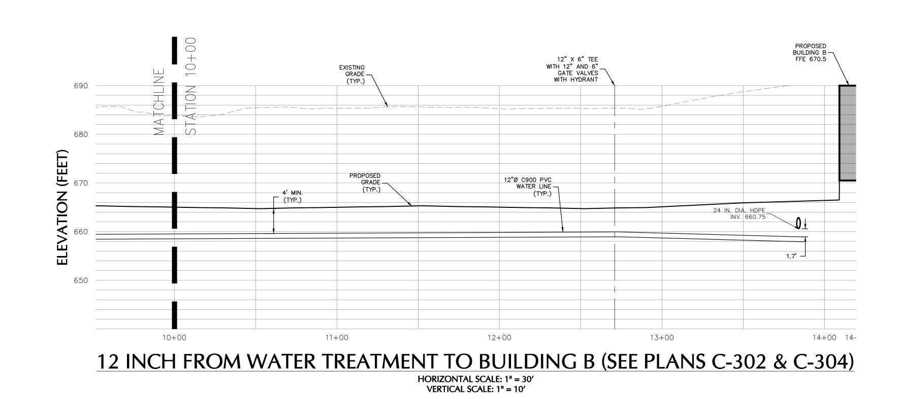
1. UNLESS OTHERWISE SPECIFIED, PIPE FOR WATER SUPPLY AND DISTRIBUTION LINES SHALL BE POLYVINYL CHLORIDE PRESSURE PIPE (PVCP), CLASS 235 PSI, DR 18, WITH PUSH—ON JOINTS IN ACCORDANCE WITH AWWA C—900 (BLUE BRUTE).
