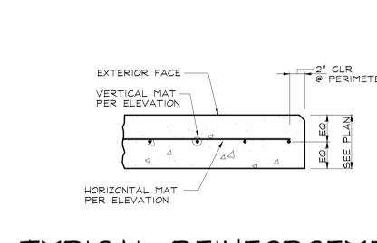
**TYPICAL REINFORCEMENT SECTION AT PANEL WITH 1 LAYER OF STEEL**
