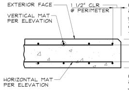
**TYPICAL REINFORCEMENT SECTION AT PANEL WITH 2 LAYERS OF STEEL**
