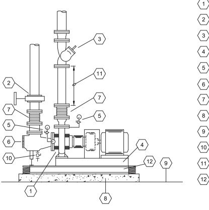
$\langle 8 \rangle$  6" CONCRETE BASE  $\langle 9 \rangle$  FINISHED FLOOR (10) 1" BALL VALVE
