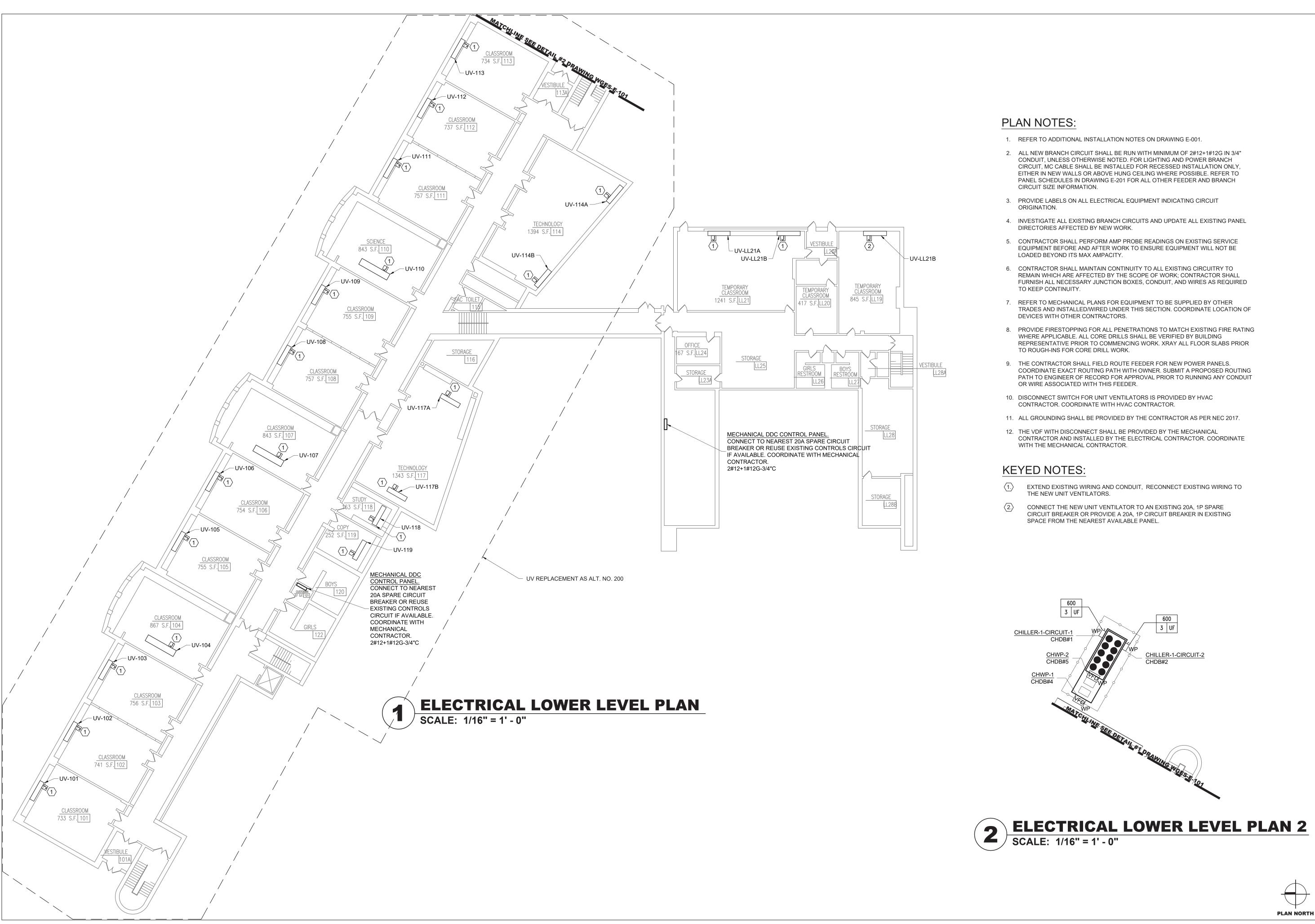
CONDUIT, UNLESS OTHERWISE NOTED. FOR LIGHTING AND POWER BRANCH CIRCUIT, MC CABLE SHALL BE INSTALLED FOR RECESSED INSTALLATION ONLY, EITHER IN NEW WALLS OR ABOVE HUNG CEILING WHERE POSSIBLE. REFER TO PANEL SCHEDULES IN DRAWING E-201 FOR ALL OTHER FEEDER AND BRANCH
