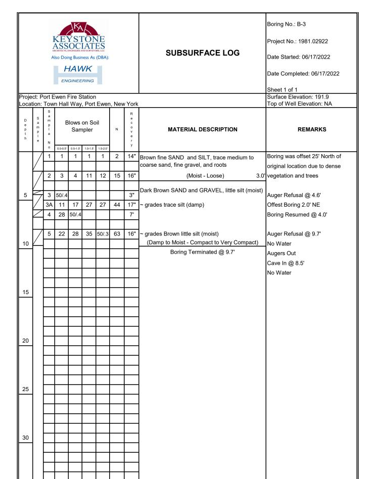
Sampling Method: ASTM D-1586, unless otherwise noted. Visually Classified by: Geotechnical Engineer Notes: 3-1/4" Hollow Stem Augers, CME 45B Drill Rig, Christiansen NWD4 Core Barrel, water as flushing medium.
