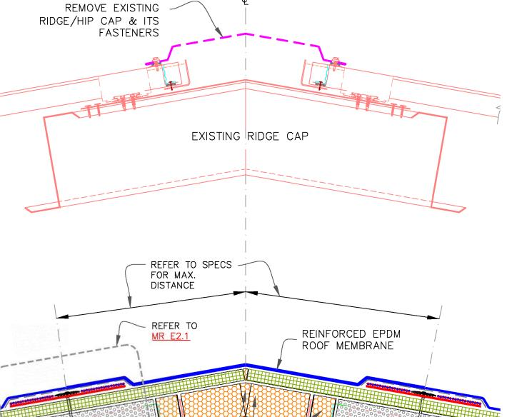
FILL WITH RIGID BOARD FASTEN TO TOP INSULATION OR INJECT PURLIN ON EACH HIGH-RISE FOAM SIDE AS SHOWN RETROFIT RIDGE CAP
