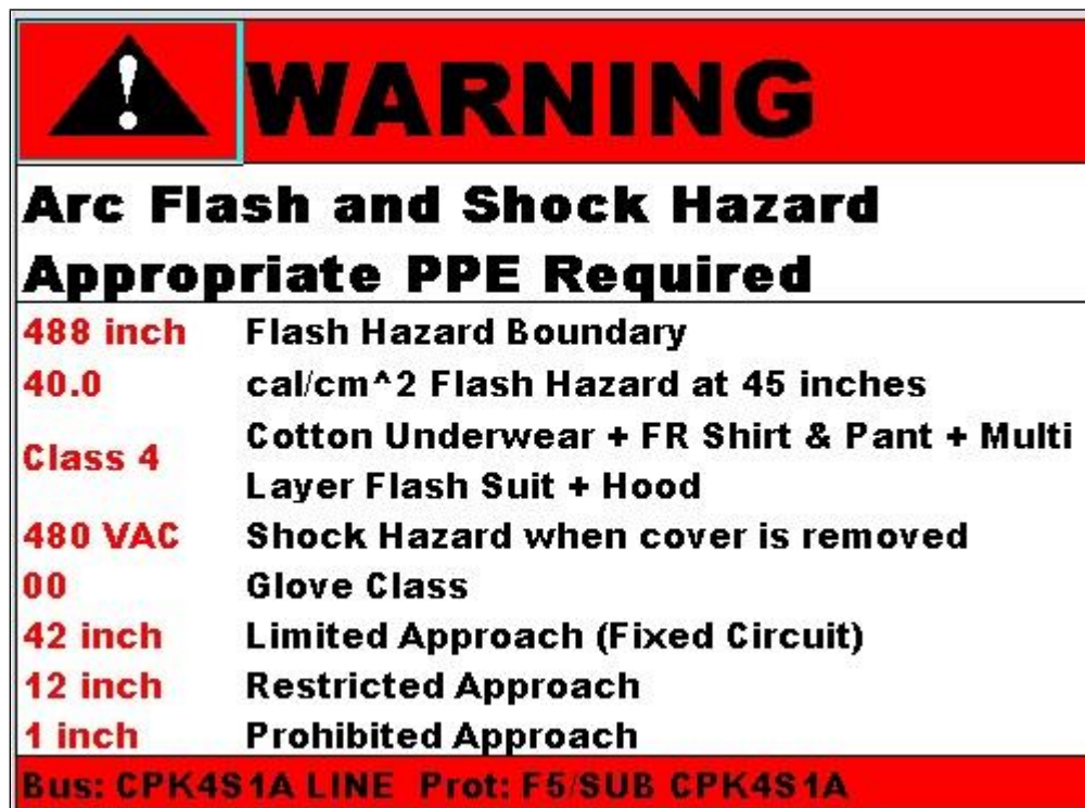
Example of Arc Flash Warning Label
