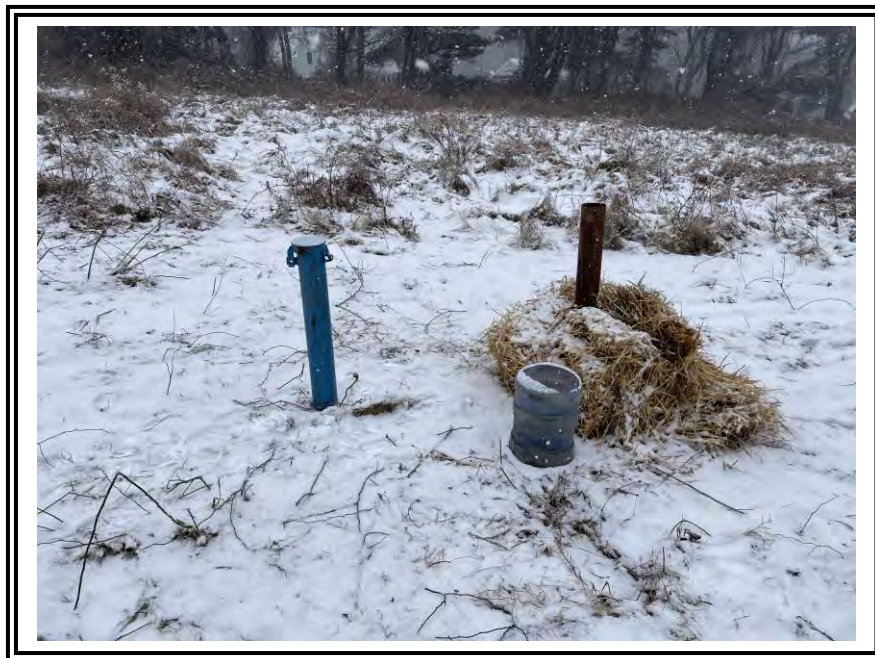
Groundwater observation well and infiltration casing installed at boring B-6A, looking west
