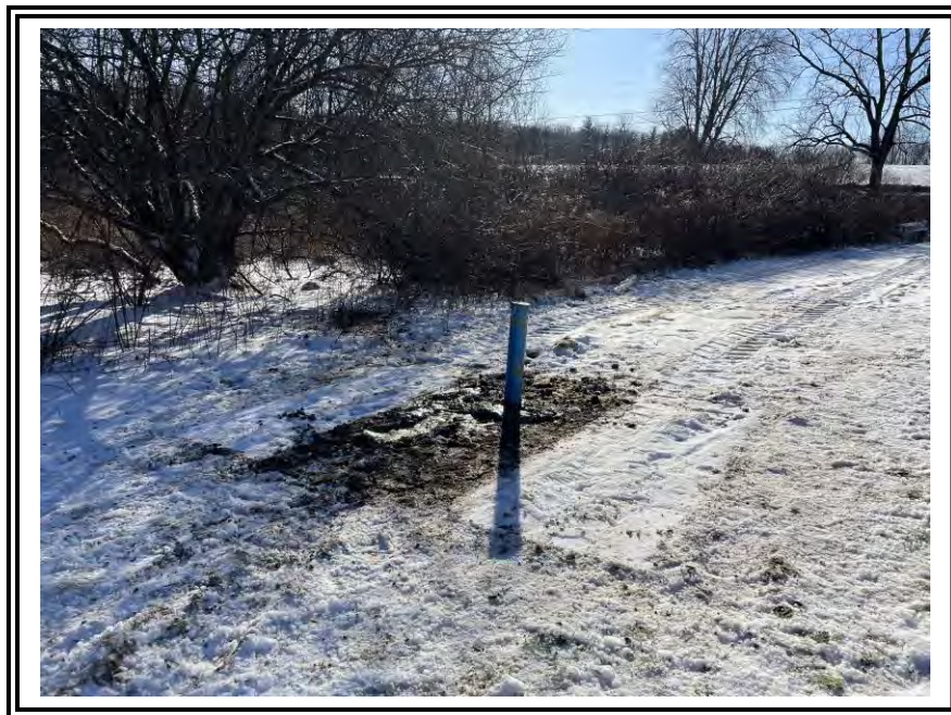
Groundwater observation well installed at boring B-10, looking southeast
