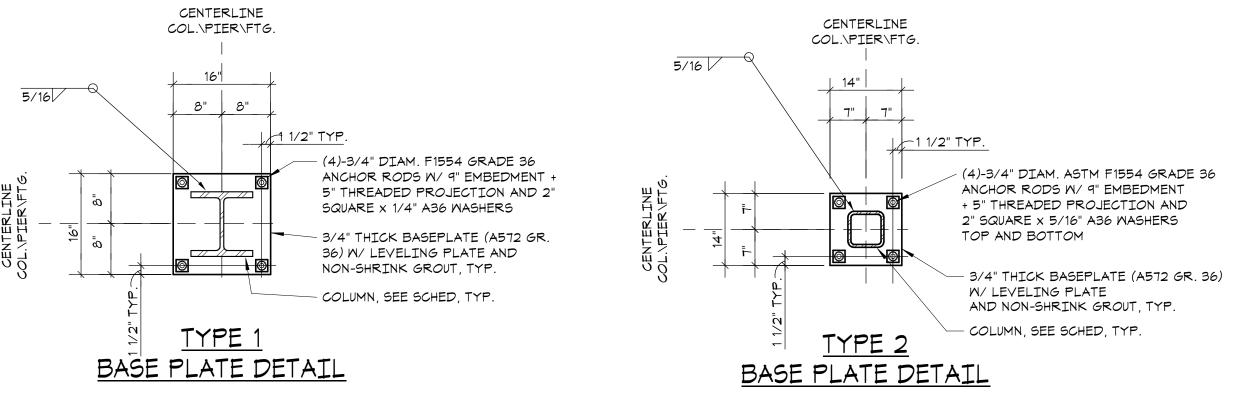
TYPICAL STEEL COLUMN BASE PLATE DETAILS
