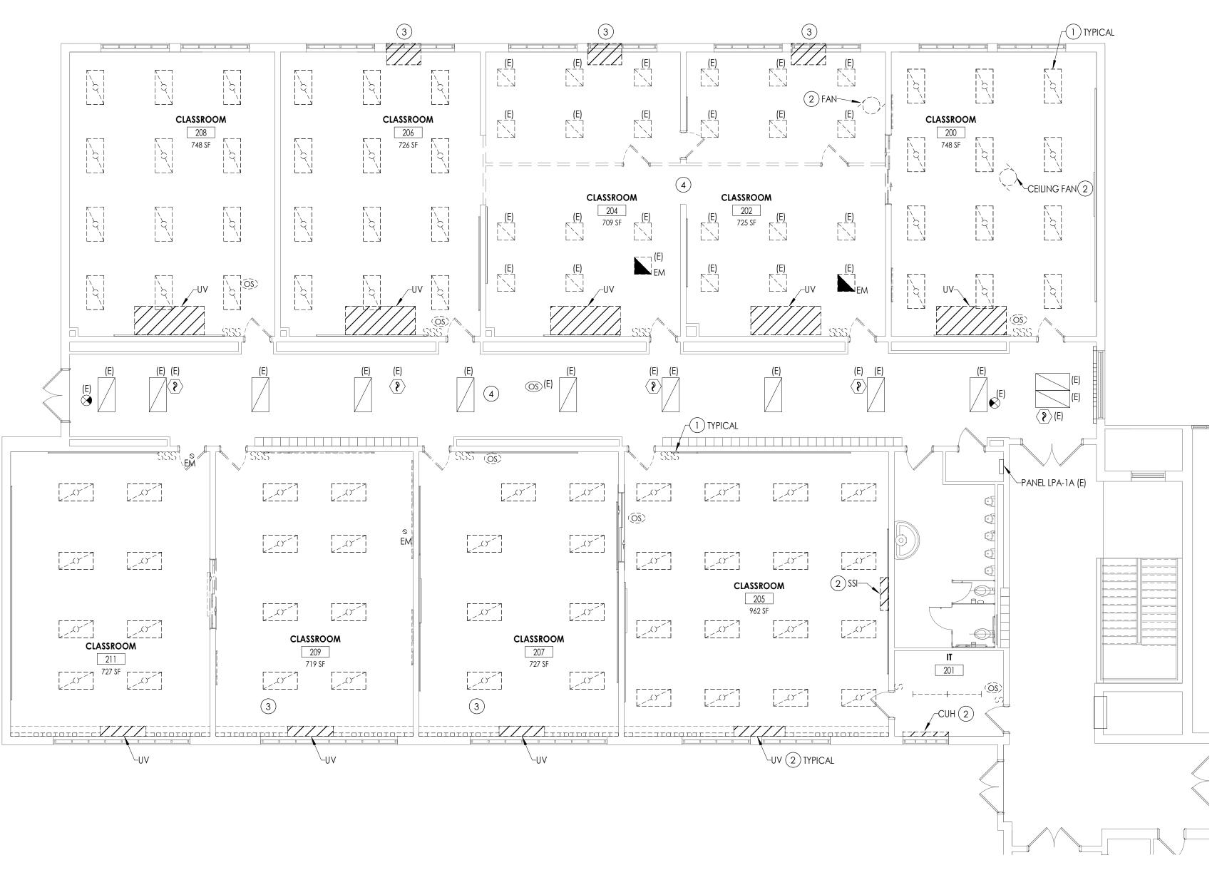
FIRST FLOOR ELECTRICAL DEMOLITION PLAN - AREA B E101 1/8" = 1'-0"
