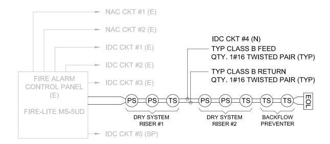
PARTIAL FIRE ALARM RISER DIAGRAM
