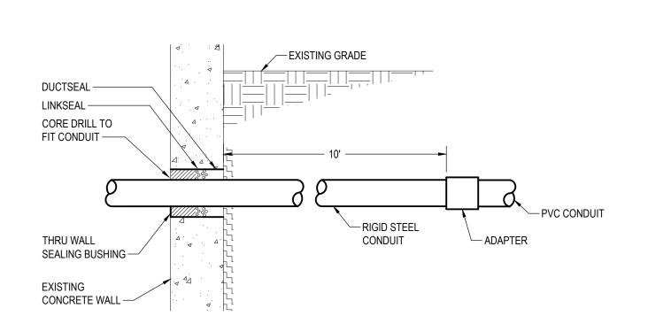
UNDERGROUND CONDUITS ENTERING EXISTING BUILDING WALL SCALE: NOT TO SCALE
