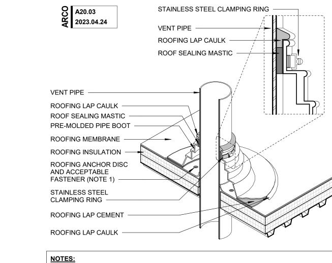
WITH MECHANICALLY FASTENED SPEC. MEMBRANE MUST BE MECHANICALLY ATTACHED WITH T.P.O. ANCHOR DISC WITH ACCEPTABLE FASTENERS (6" [150mm] CENTERS AROUND PIPE VENT) DO NOT OVERLAP THE FLANGÉS FROM ADJACENT PIPE FLASHING. ANY SEAM UNDER BOOT FLANGE TO BE TREATED AS T-JOINT
