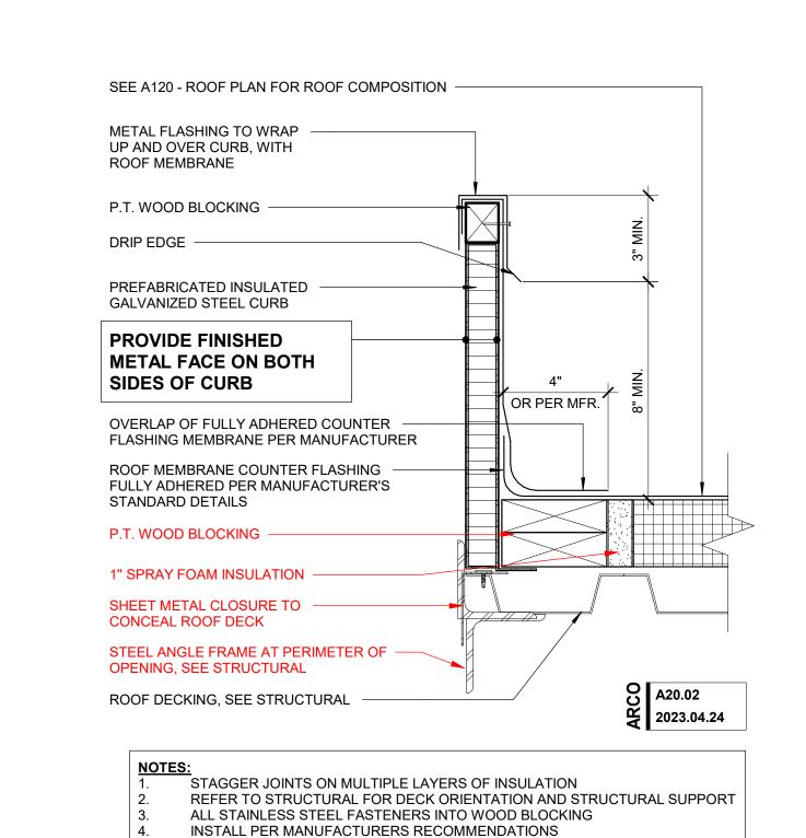
**ROOF MECHANICAL CURB** SCALE: 3" = 1'-0"
