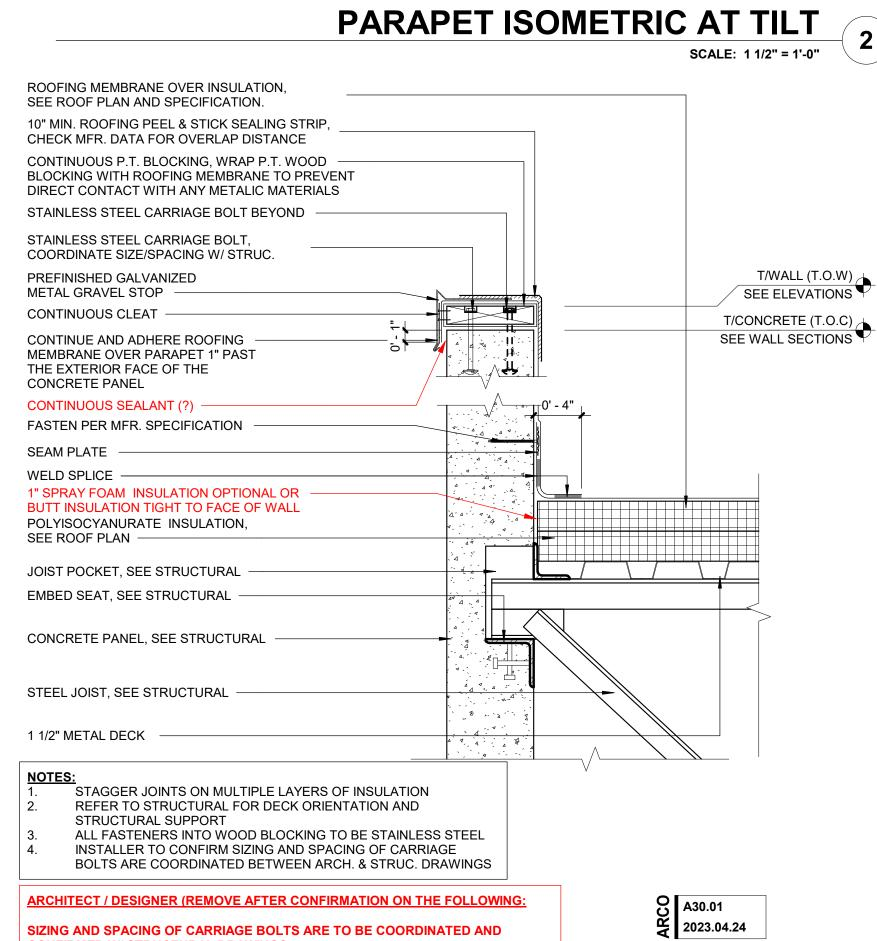
SIZING AND SPACING OF CARRIAGE BOLTS ARE TO BE COORDINATED AND
