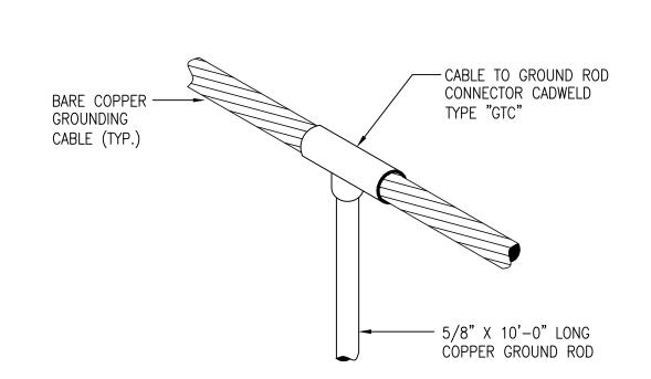
CONTINUOUS CABLE TO GROUND ROD CONNECTION SCALE: NONE
