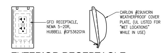
EXTERIOR RECEPTACLE DETAIL SCALE: NONE
