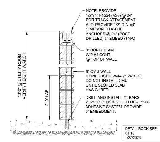
INTERIOR MASONRY WALL SCALE: NO SCALE
