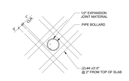
S1.08 1/27/2023 REBAR @ PIPE BOLLARDS SCALE: NO SCALE
