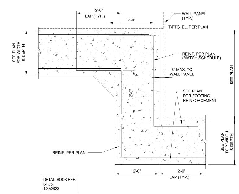
SECTION AT FOOTING STEP SCALE: NO SCALE
