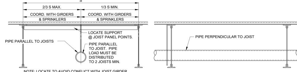
NOTE: LOCATE TO AVOID CONFLICT WITH JOIST GIRDER. PIPE PARALLEL TO JOISTS
