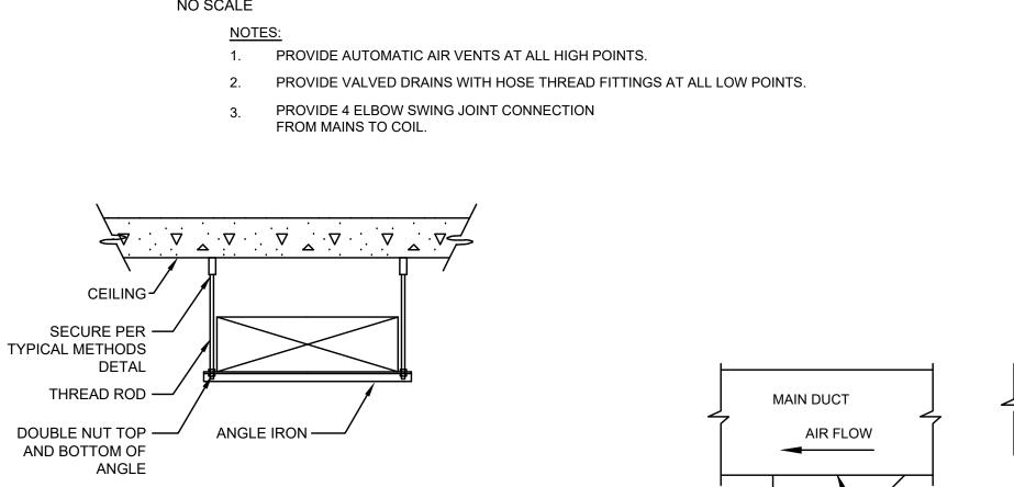
CONTRACTOR SHALL PROVIDE ADDITIONAL SUPPORTS AS NECESSARY
