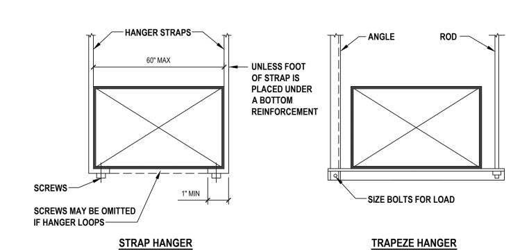
1. SIZE ALL SUPPORTS IN ACCORDANCE WITH THE SMACNA DUCT CONSTRUCTION STANDARDS, LATEST EDITION.
