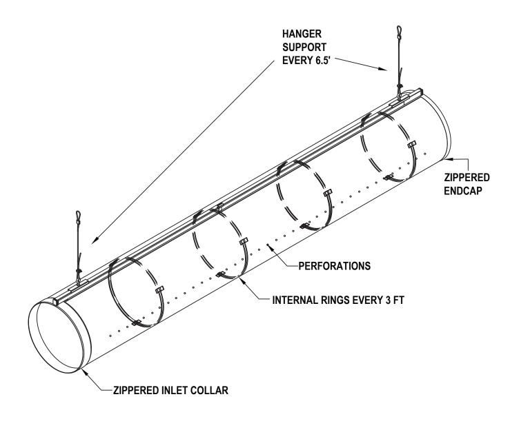
6 Fabric Duct Installation Detail
