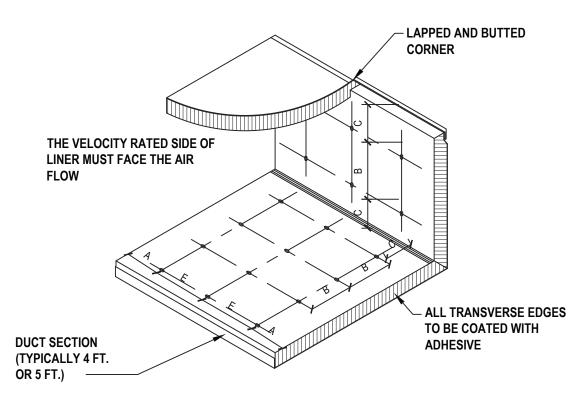
MAXIMUM SPACING FOR FASTENERS. LINER ADHERED TO THE DUCT WITH ACTUAL INTERVALS ARE APPROXIMATE. 90% MIN. AREA COVERAGE OF
