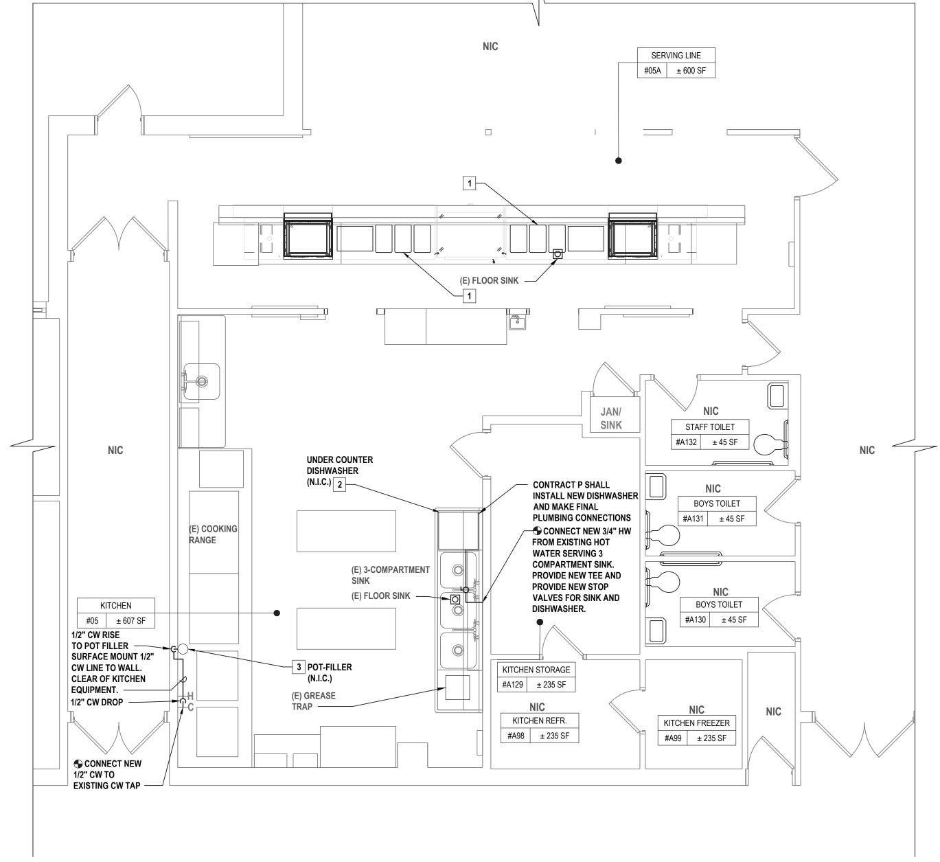
**EXAMPLE 2** Kitchen & Serving Line Construction Plan SCALE: 1/4"=1'-0"
