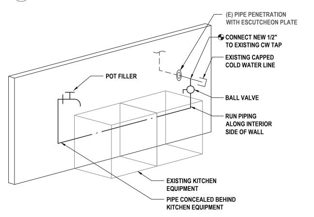
9 Pot Filler Plumbing Routing Detail
