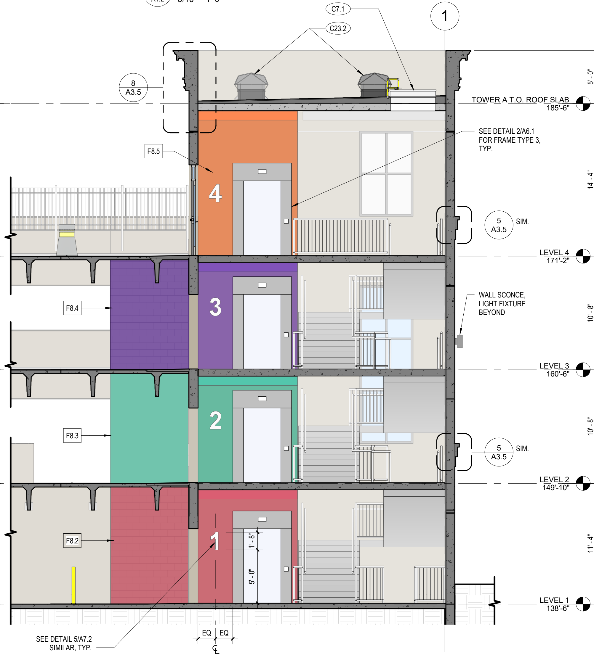
5 STAIR/ELEVATOR TOWER A SECTION/ELEVATION LOOKING EAST 3/16" = 1'-0"
