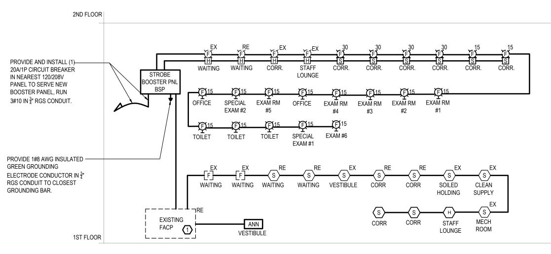
PARTIAL FIRE ALARM WIRING DIAGRAM NOT TO SCALE
