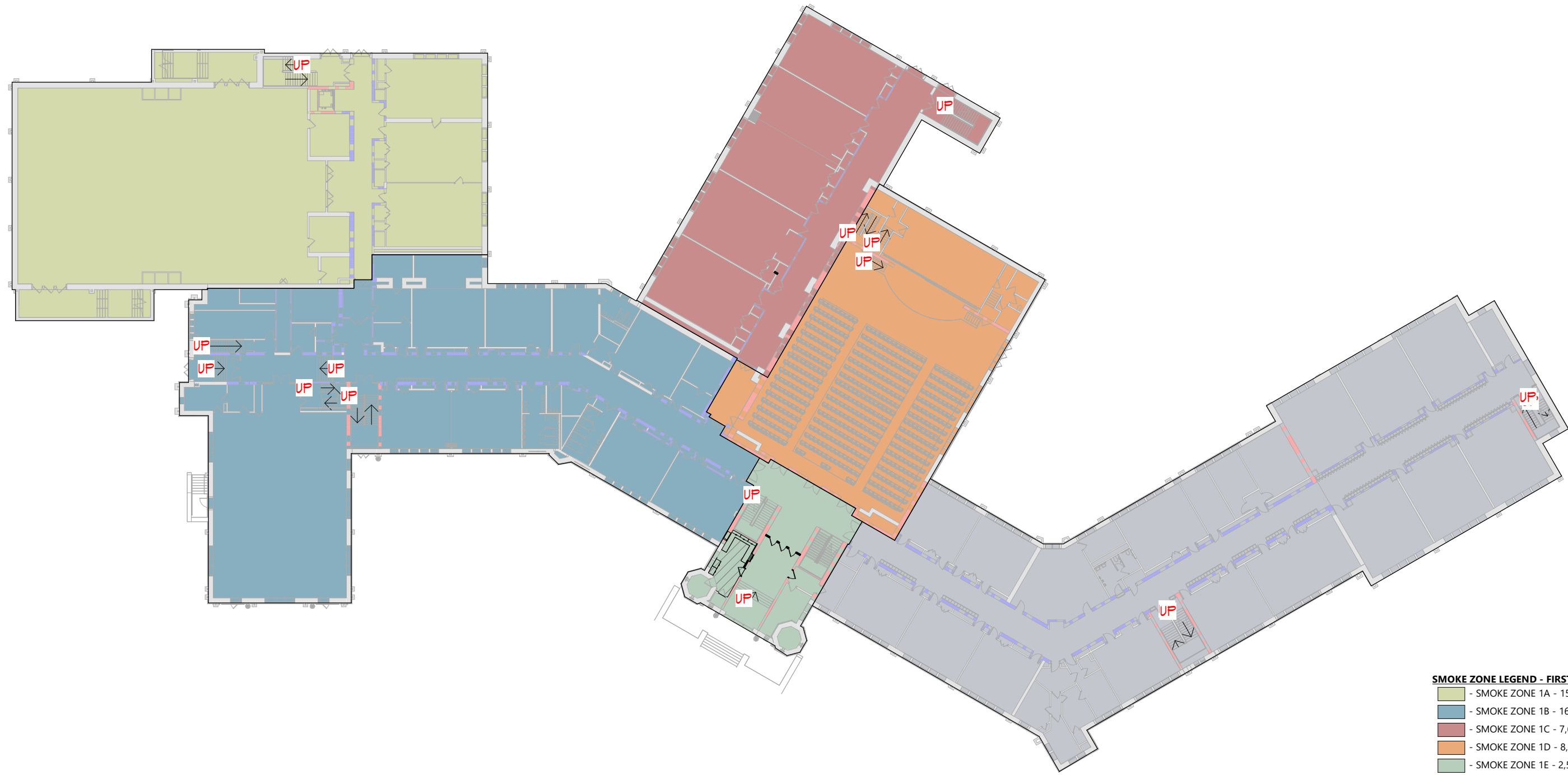
2 FIRST FLOOR SMOKE ZONE PLAN LS124 1" = 40'-0"
