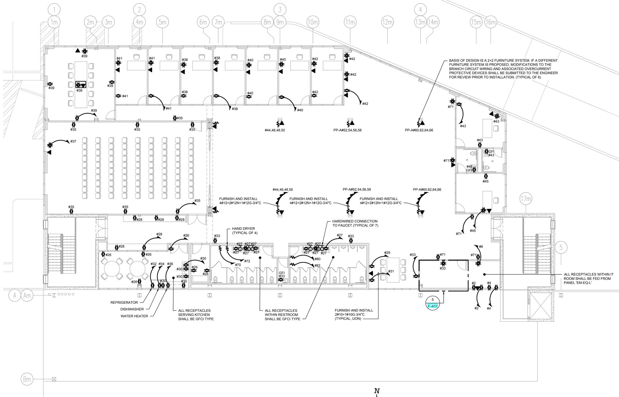
BASIS OF DESIGN IS A 2+2 FURNITURE SYSTEM. IF A DIFFERENT FURNITURE SYSTEM IS PROPOSED, MODIFICATIONS TO THE BRANCH CIRCUIT WIRING AND ASSOCIATED OVERCURRENT PROTECTIVE DEVICES SHALL BE SUBMITTED TO THE ENGINEER FOR REVIEW PRIOR TO INSTALLATION. (TYPICAL OF 6)
